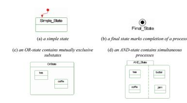
Hierarchy (i.e. substatechart) is made possible by: the "OR-state" Figure 3(c) which includes exclusive substates inside a parent "OR-state" and the "AND-state" Figure 3(d) which allows concurrent processes to run simultaneously. The concurrent processes of the "AND-State" are graphically divided by dashed lines.
