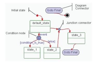
*Figure 4. Pseudo-states (initial state, condition, junction and fork as well as "diagram connectors") are useful graphical abbreviations*
